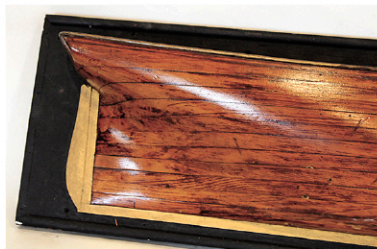
Stern of half hull, Length: 5' with 10 lifts
