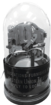
RC2174. Edison model 32A stock ticker with glass dome and ticker tape. 14"H x 9"Dia
