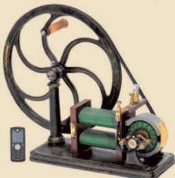
Large Current Generating Dynamo, c. 1910
