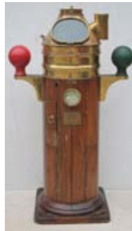
Fine ca 1900 mahog & brass w iron compensating balls 55" tall marine binnacle by Kelvin & Hughes w WWII compass by The Lionel Corp dated 1942
