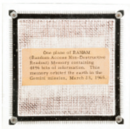
Gemini 3: Flown Random Access Non-Destructive Readout 4096 Bit Memory Plane. Sold for $20,000
