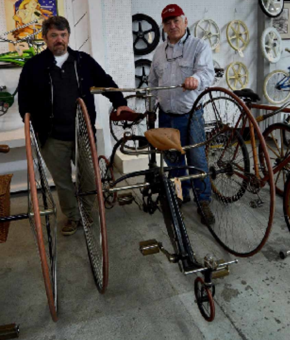
Auctioneers Seth and Mike Fallon show off the 1886 Singer "The Traveller Tandem," made in Coventry, England ("Humbers Patent"). Singer had a license from Humber and the bike's front part is quickly detachable leaving a Humber-type single machine when desired. The bicycle sold for a reasonable $10,237.
