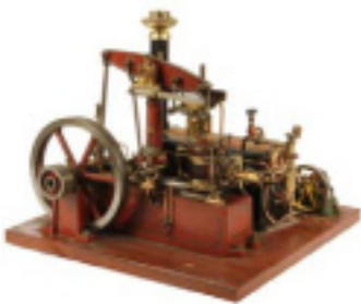
Lot 1268 - Stuart Steam Model of Watts Double-Action Beam Engine with 7" flywheel, 1" bore, 2" stroke, Circa 1925. 14" x 16" x 16". est. $2000 - $3000
