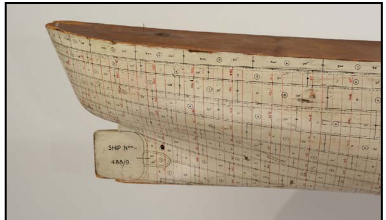
JUDITH & JAMES MILNE, Kingston, N.Y. — Half-hull plating model, 6 feet 4 inches, retaining its original graphic detail.
